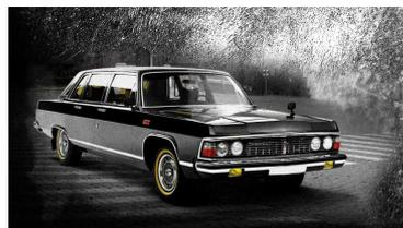
Also known as the Chaika ("Seagull"), it was considered the height of luxury at the time: with a push-button automatic transmission, 8-cylinder engine, 220hp and a top speed of 99mph.
